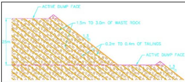
Figure 6 Layering of tailings on the dump face
